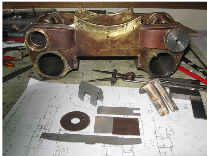
Photo shows cylinder block under construction, with valve spindle guides, one in pieces before assembly.
